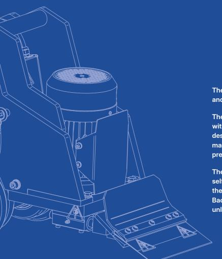
The machine works under its weight on the floor and it is to be led by an operator.
