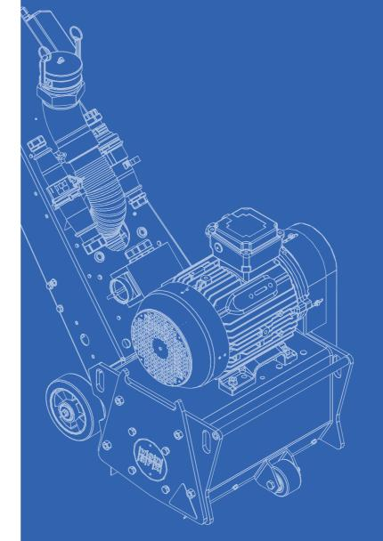
Ideal where paved surfaces need to be roughened, grooved, cleaned, or where layers need to be removed. The VA 30 S' infinite variable depth adjuster allows to adapt perfectly to every surface.
